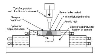
**Figure 1** Schematic illustration of the sample positioned on the apparatus for alignment and application of load in the Universal testing machine.
